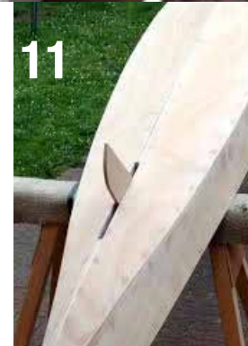
5. Inwhale fitting 6 Hull stitched 7. Taped seams 8. Masik jig 9. Mask in place 10 Foredeck fitted 11. Skeg fitted
