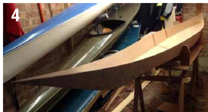
1. Plans transferred. 2 Cut panel 3. Bow stitching 4. Stitched hull
