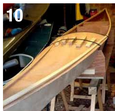
5. Inwhale fitting 6 Hull stitched 7. Taped seams 8. Masik jig 9. Mask in place 10 Foredeck fitted 11. Skeg fitted
